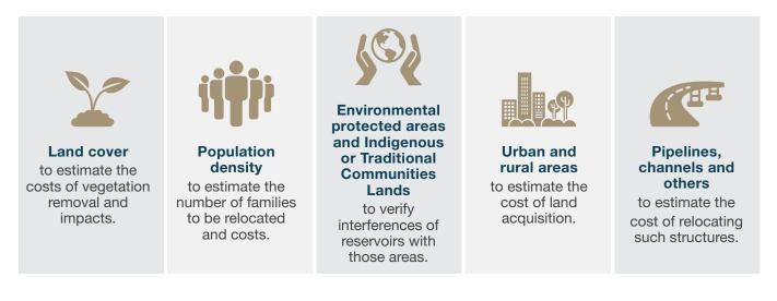
**HERA** computes the intersections between reservoir flooded area and layers of user provided information (i.e. shapefiles) to determine costs related to environmental aspects and constraints. For each site, different options can be studied by varying the head and engineering layouts. A plant scheme of each project with estimated costs and installed capacity can be visualized.
